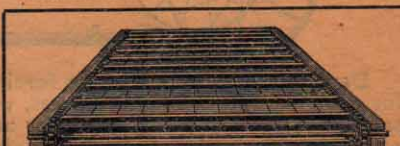
Bottom of David Bradley Spreader, showing endless steel apron, with No. 62 malleable chains and angle steel protecting tracks underneath. Note the watertight floor and heavy side sills.
