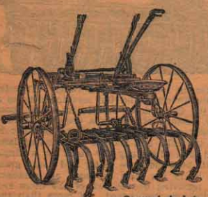
Converted into a riding spring tooth harrow by using center attachment.
